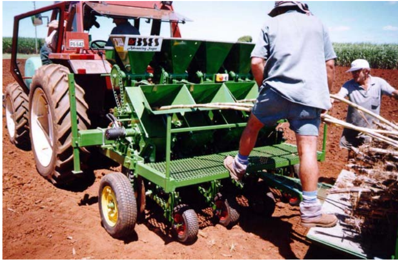
Figure 20. Multi-row whole-stick planter in operation
