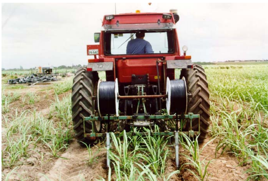
Figure 30. Trickle-tape installer for four rows on 2.1-m beds
