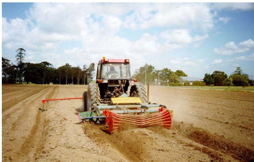
Figure 19. Bed former and tactile guidance system in operation
