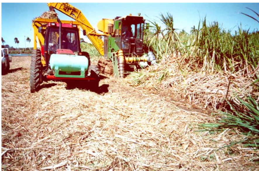
Figure 31. Multi-row harvester and haulout cutting cane - Qunaba trial 2000. Average yield from 2.1-m beds was 245 tonnes cane per hectare
