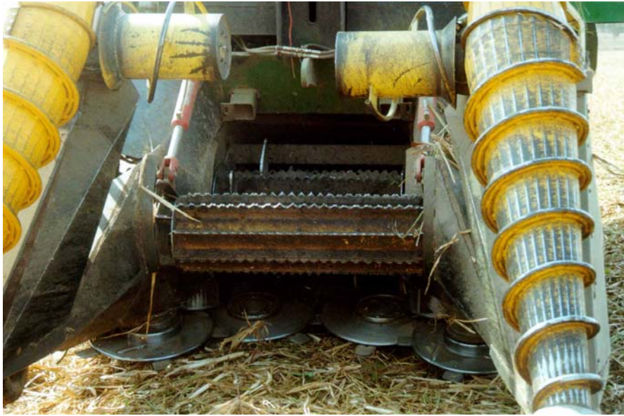
Figure 32. Four base cutters and spirals fitted to the multi-row harvester (August 2002)
