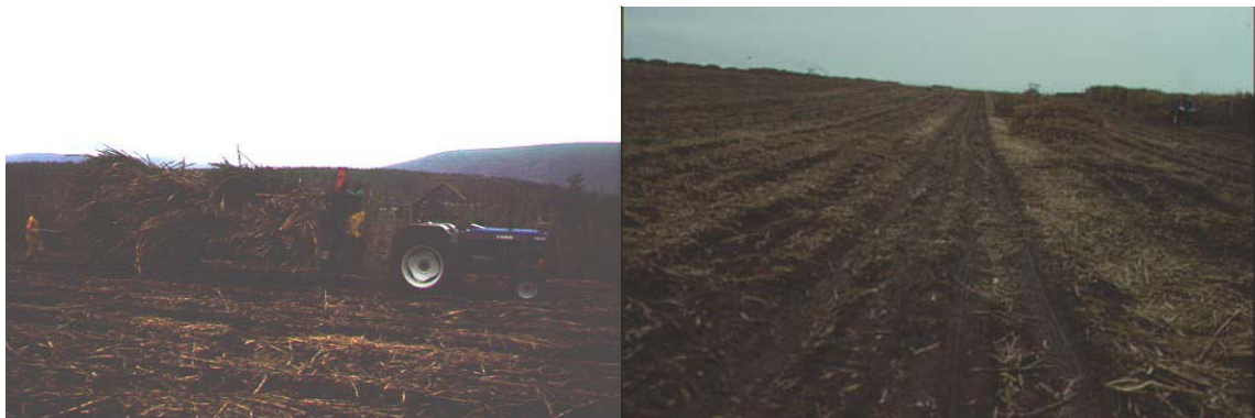
Figure 6. (Left) Winch-loaded trailers at Big Bend in Swaziland; (Right) Compaction of traffic lanes from winch trailers
