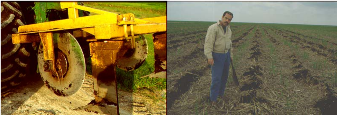
Figure 7. (Left) Coultter ripper at Osceola Farms, Florida; (Right) After passage of coultter ripper where the leg penetrated to the full depth of the cane knife blade.
