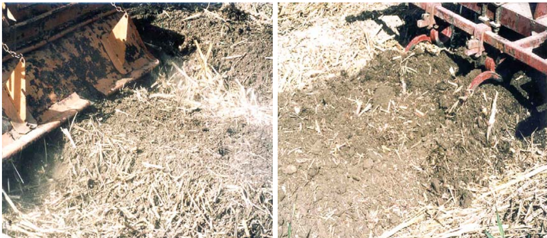
Figure 2 Shallow rotary hoeing and ripper tine operation in strategic tillage
