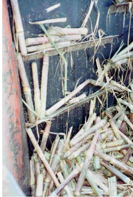
Figure 64 Rubber belt elevating conveyor showing two rows of offset slats and number of billets conveyed per slat
