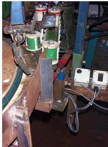
Figure 74 Ribbed metering belts showing modified flipper and control box for billet feed onto the disc
