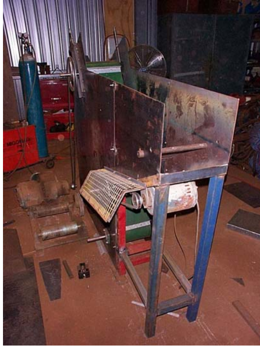
Figure 71 Prototype vibrating billet-alignment system
