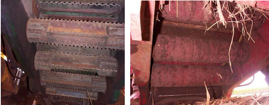
Figure 28 Feedtrain rollers: (left) commercial steel rollers; (right) modified rubber-coated rollers
