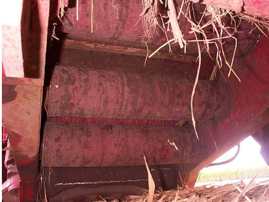
Underside view of rubber coated rollers on Austoft 7000
