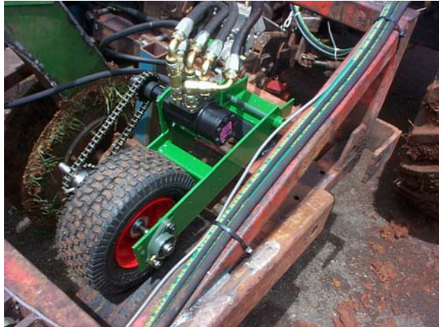
Figure 79 Hydraulic ground-drive system controlling billet metering rate showing jockey wheel and hydraulic metering valve
