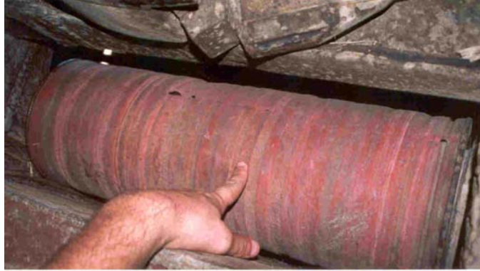
Figure 29 Grooves in a rubber-coated roller caused speed mismatch
