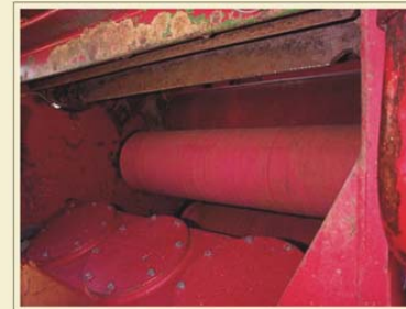
Rubber coated rollers fitted to the top roller group of an optimised harvester.
