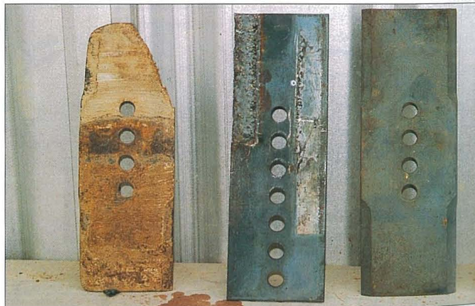
LEFT: Worn blade — increases stool damage and soil intake. Centre: Hard surfaced blade. Right: Reversible blade.
