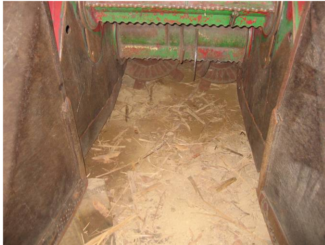
Figure 6 Modified front for harvesting dual-row cane
