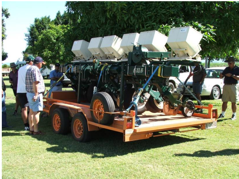
Figure 2 Disc-opener legume planter at BSES Mackay
