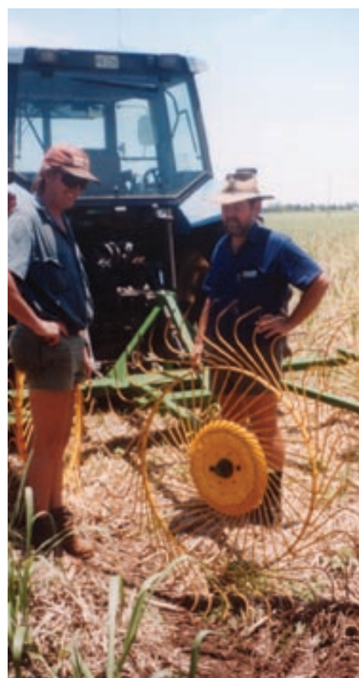
Bottom: Trash is easily removed from the irrigation path with a finger wheel rake.
