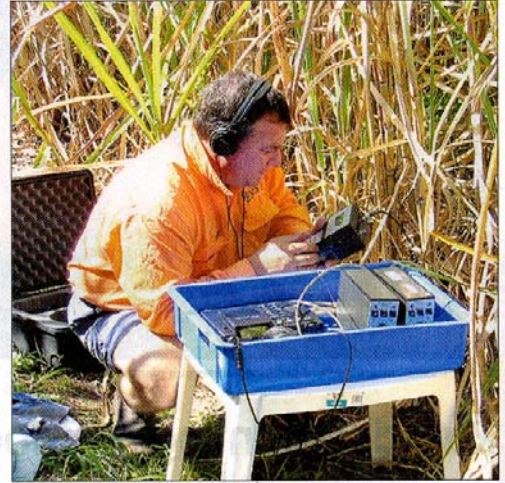
AMERICAN developed detection equipment listens in to cane grub activity on a central district farm. Picture: Contributed
