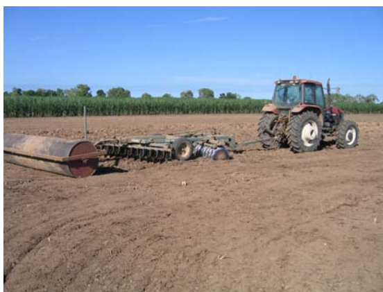
Figure 12 Secondary cultivation was achieved with off-set discs and a roller.
