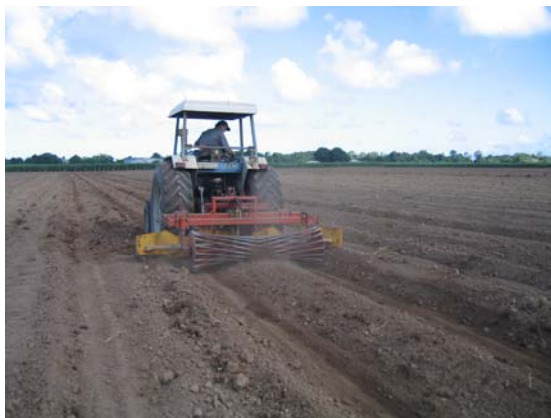
Figure 13 Preformed mounds were established using a single-row bed former.
