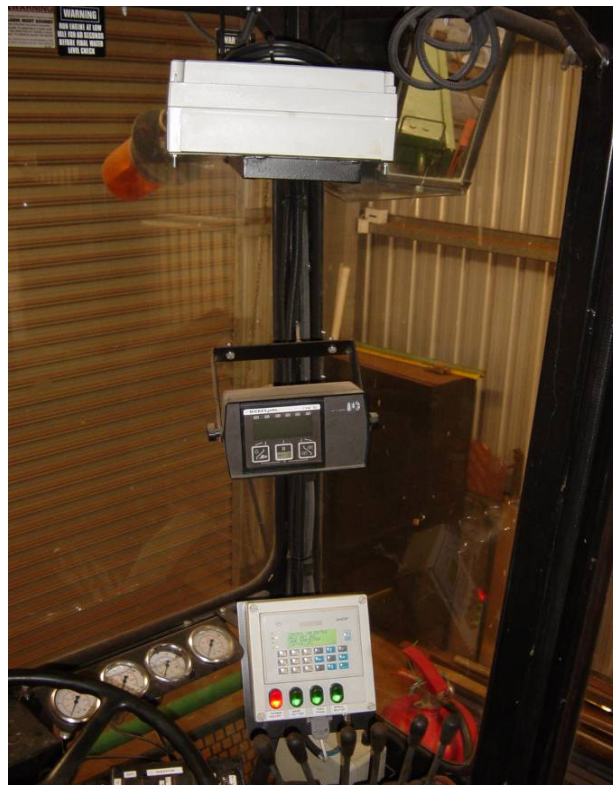
Figure 48 Automated speed control system as installed in harvester cab showing: PLC interface between component speed sensors and the electric-over-hydraulic controllers (top box), the Dickey-John radar ground speed display (middle) and the operator feedback console (bottom box) as installed inside the harvester cabin
