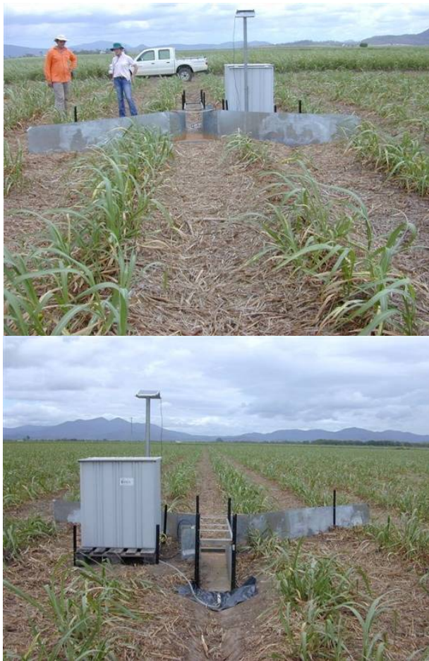
Figure 20 Water samplers set up at Gerry Deguara's farm
