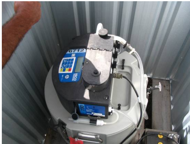
Figure 23 Isco water samplers installed at the Marian site
