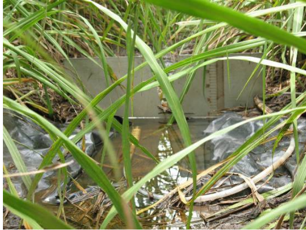
Figure 24 Sampling weir installed at the Farleigh site
