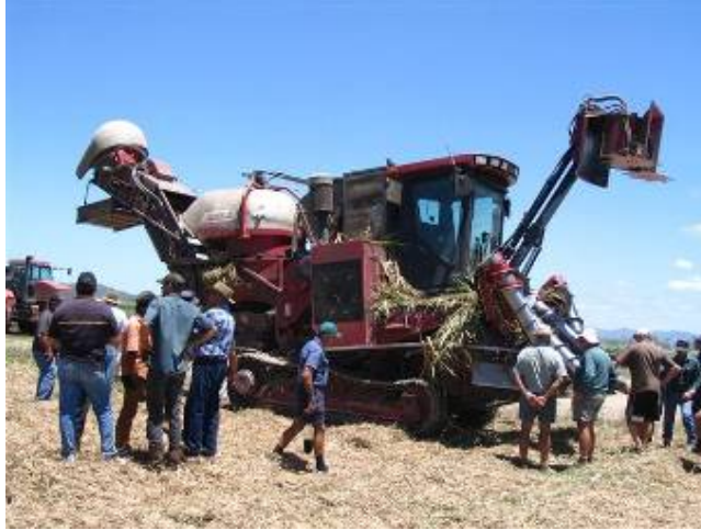
Figure 2 Growers examining Bruce Davies's harvester during the bus tour. Note the elevator extension used to harvest 1.8 m rows
