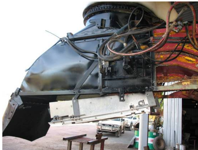
Figure 11 New aluminium elevator extension
