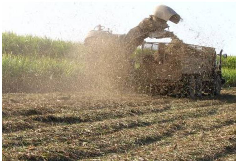
Figure 18 Harvesting the trial at Jim Sivers' farm. Note the lodged cane in the foreground and the standing cane in the background. The lodged cane is the 1.83 m dual rows and the standing cane is the 1.83 m single rows. Also note the NFS harvester elevator extension used on the harvester to allow the haulout to remain on the wheel tracks.
