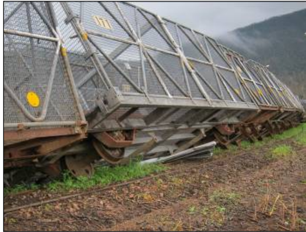
4 Feb 2011 – Cane bins blown off tram line at Tully Mill
