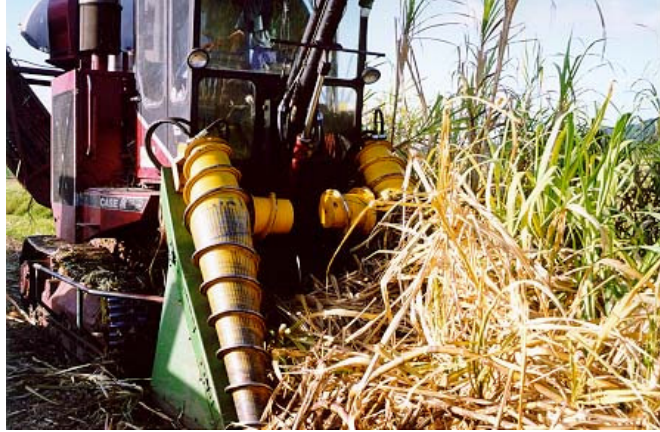
Plate 1 - BSES modified fronts on Austoft 7700 harvester The harvester is operating in a 160 t/ha crop of Q124
