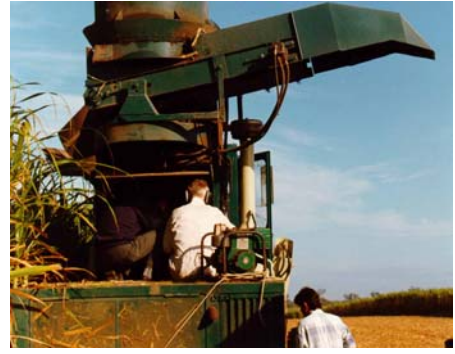
Photo 4 - View of rear of harvester showing the position at the back of the machine from which filming occurred. The portable alternator is to supply power for supplementary lighting.
