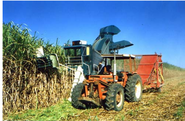
Photo 2 - Bonel Chop-Throw harvester prototype which was used in the investigation
