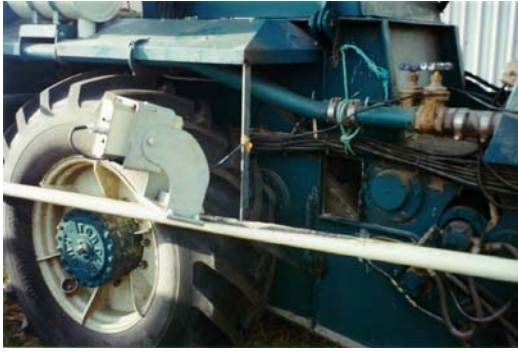
Photo 3 - View of high-speed camera and viewing window adjacent to the thrower and rotary anvil.
