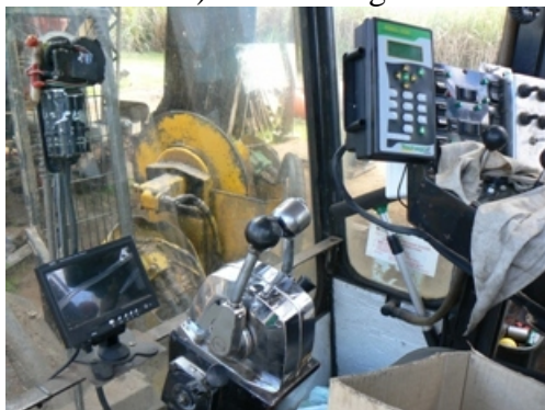
Figure 17-External camera fitted. Figure 18- Camera screen in the cabin.
