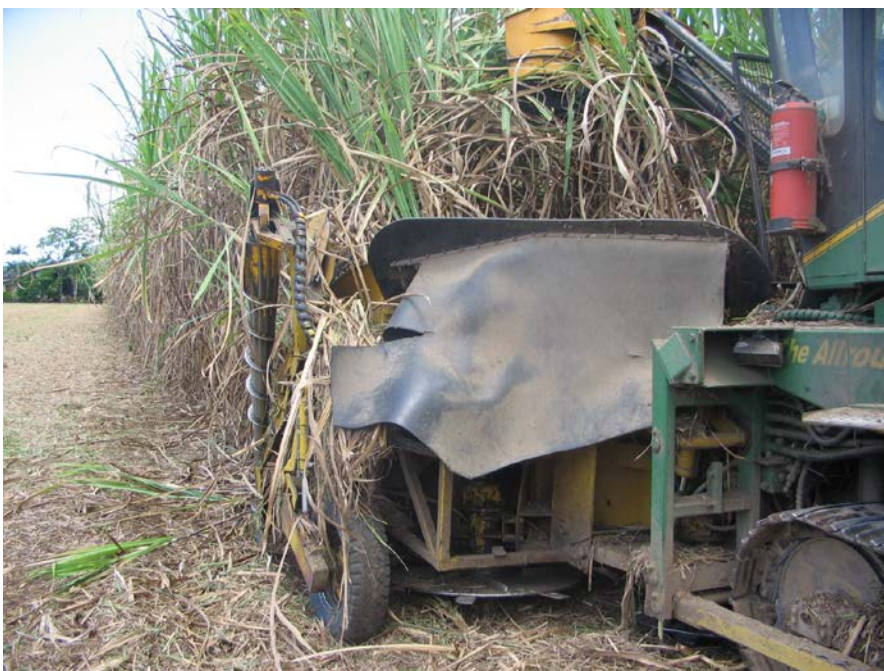
Figure 7. The Two in One unit harvesting 1.64m rows
