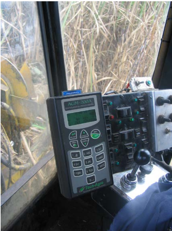
Figure 1 shows the on-board computer installed in the harvester.
