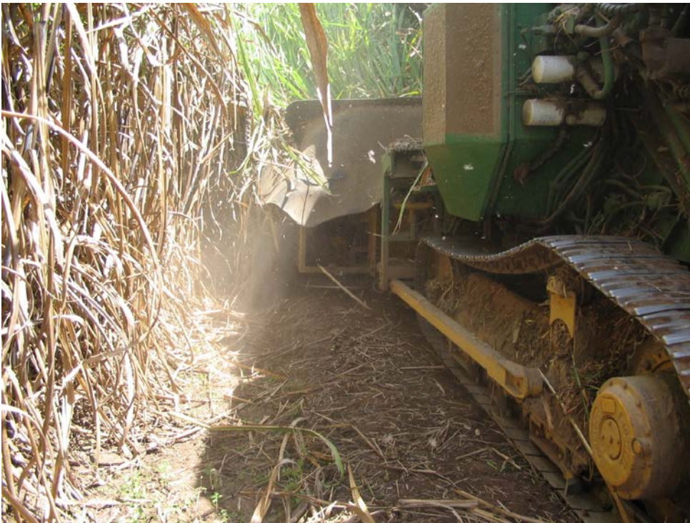
Figure 19. Harvesting of 1.85m rows in automatic function on the Two in One.
