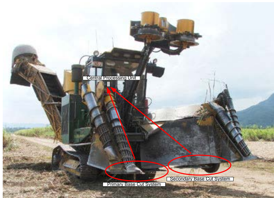
Figure 4. Hardware components in the harvester
