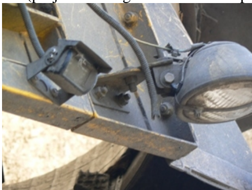
Figure 17-External camera fitted. Figure 18- Camera screen in the cabin.
