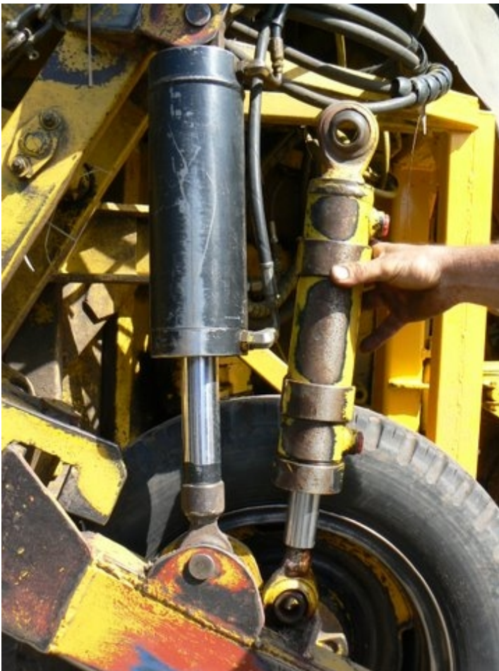
Figure 11. Comparing the new and old hydraulic lifting rams.
