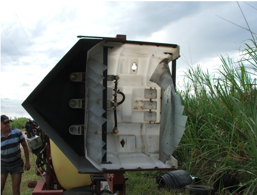
Figure 1. After modifications the three sensors sit outside the spray chamber.
