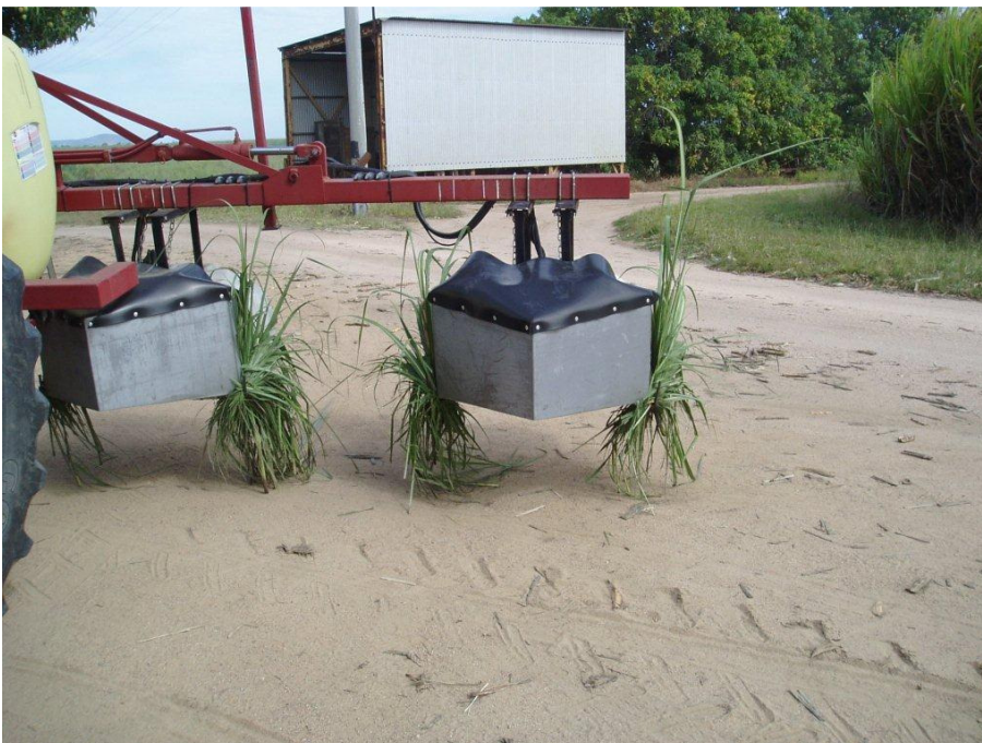
Figure 4. Cane leaves caught by crop defectors, caused the sensors to spray herbicide unnecessarily.
