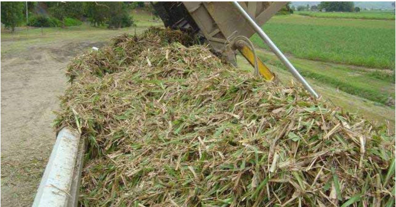
With the amount of biomass product required to achieve above 21tonne payload target the road transport bin needed to be loaded 500-600mm above the sides.
