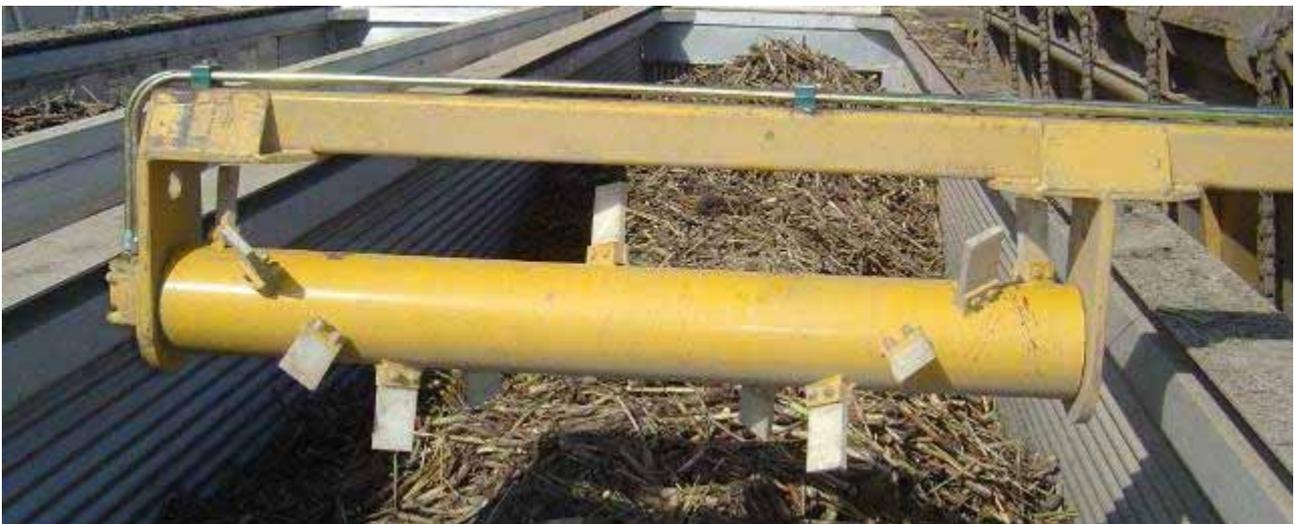
A roller configuration consisting of three blades the roller width of each blade made of two strips flat steel 40mm apart at bottom mounting point and together at the apex was tried.
