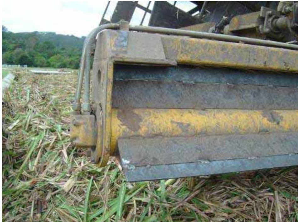
This configuration proved excellent for two applications. First when matching ground speed and rotation directing the arm worked as an effective roller compacting product improving bulk density with first pass, then on second pass the rotation is reversed and the arm moved the product out in front levelling the product, each pass was completed in less than 60 seconds.
