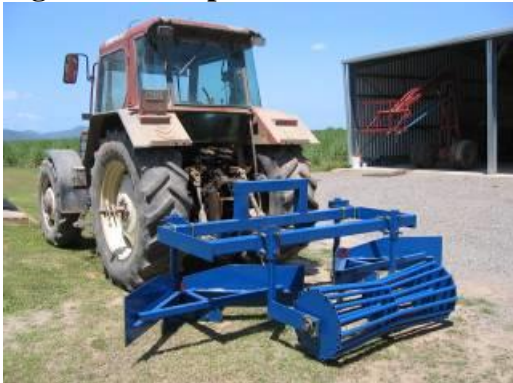
Figure 4. Completed mound former
