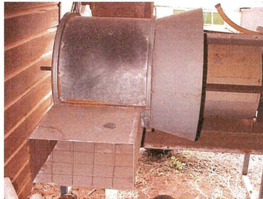
Image 16 - The tangential draw-off duct with grid wires to facilitate measurement of velocity profiles.
