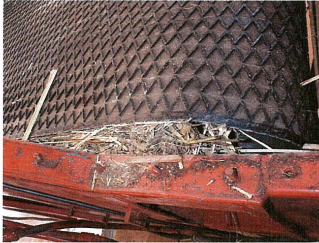
Image 28 - Belt tracking instability allowed the belts to contact the sides of the frame, causing rapid wear. This then allowed material to get between the belts as well as build up on the backing plate and rollers.
