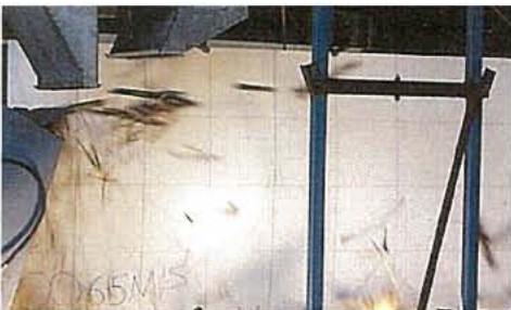
Image 14 - The trajectory of cane billets and trash from the high-speed elevator at a belt speed of 6.5 m/sec and pour rate of approximately 50 t/h with a vertical air stream of 50 m/sec and a second at 30 m/sec angled at 45 degrees, as indicated
