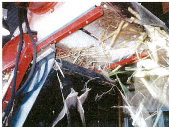
Image 30 - Test 7b. The billets and trash exit the hugger belts and pass through the air curtain, with the trash being taken down the trash chute via the induced air stream.
