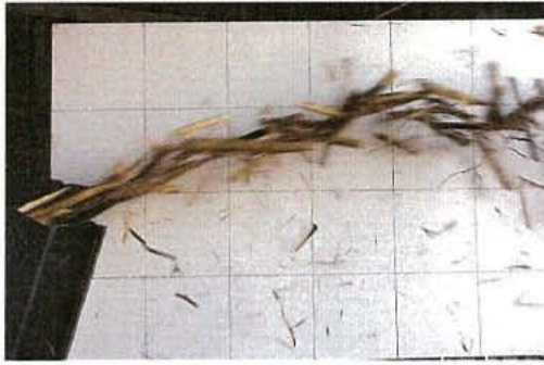
Image 11 - The trajectory of cane billets and trash from the high speed elevator at a belt speed of 6 m/sec and pour rate of approximately 70 t/h. The grid lines are at 300 mm intervals. No air flows have been introduced.
