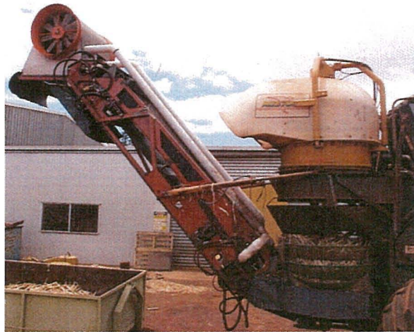
Image 27 - Overall layout of the elevator bowl, elevator and secondary cleaning system mounted on the harvester.
