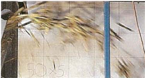
Image 12 - The trajectory of cane billets and trash from the high-speed elevator at a belt speed of 4.5 m/sec and pour rate of approximately 50 t/h with no introduced air flows.
