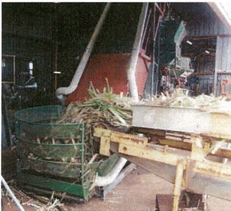
Image 29 - The elevator bowl being fed by pre-billeted whole cane. Pour rates of whole cane in excess of 100 t/h were achieved.
