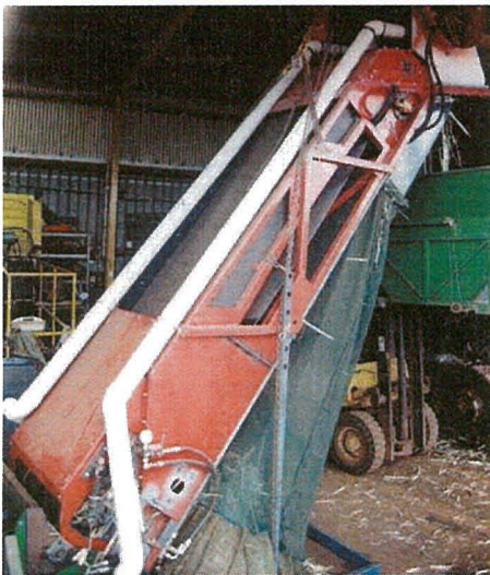
Image 26 - The elevator during workshop testing. The PVC pipes are used to duct air to between the belts to reduce trash buildup on the tail rollers. The shade cloth 'bag' collects trash from the trash duct during trials.
