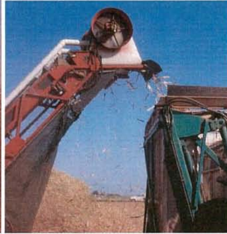
Image 32 - The shade-cloth bag on the secondary trash chute allowed trash extraction efficiency to be measured.
