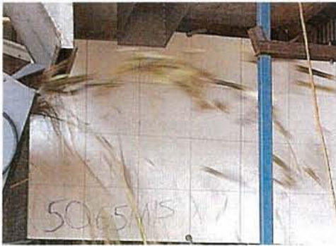
Image 13 - The trajectory of cane billets and trash from the high-speed elevator at a belt speed of 6.5 m/sec and pour rate of approximately 50 t/h with vertical air streams of 50 m/sec and 20 m/sec as indicated.
