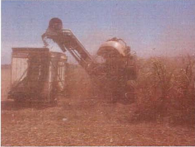
Image 31 - The high-speed elevator operating. Note the trash chute and some disturbance of trash on the ground by the air from the secondary cleaning system.
