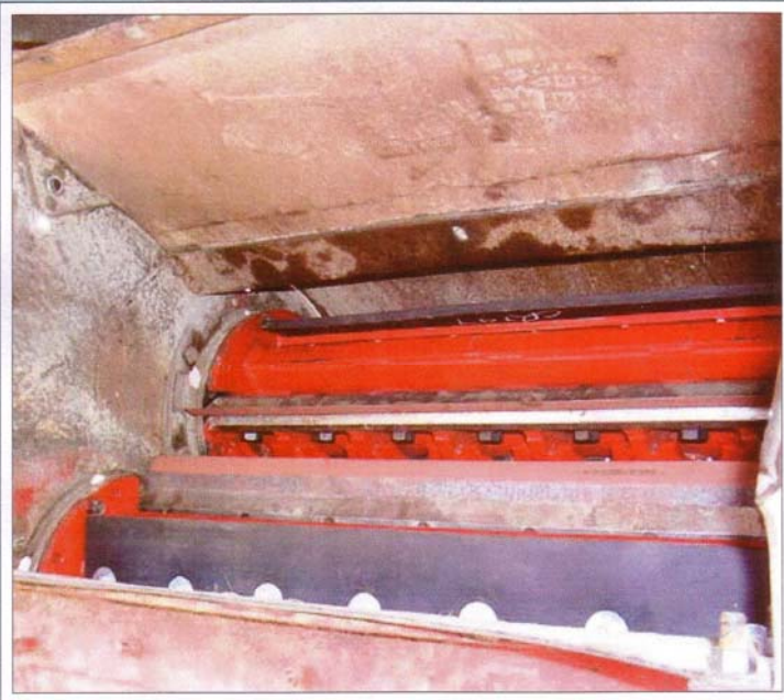
Modified rotary pinch chopper setup in an Austoft harvester.
