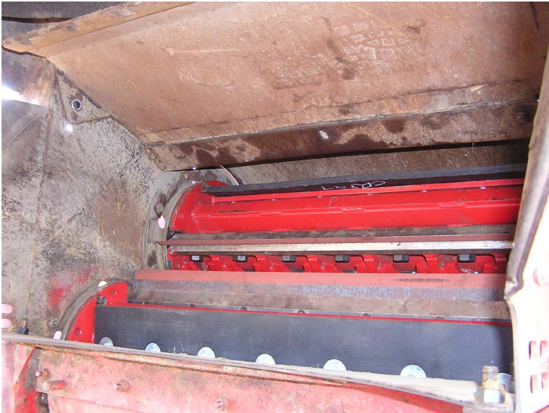
PHOTOGRAPH 5 - ‘CORRADINI’ PROOF-OF-CONCEPT MODIFIED ROTARY–PINCH CHOPPER SYSTEM INSTALLED ON 2006 TRIAL HARVESTER
