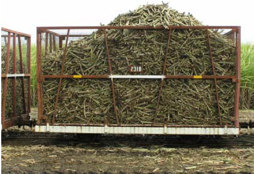
PHOTOGRAPH 12 - PILING OF MATERIAL ABOVE SIDES OF CANE RAILWAY BIN
