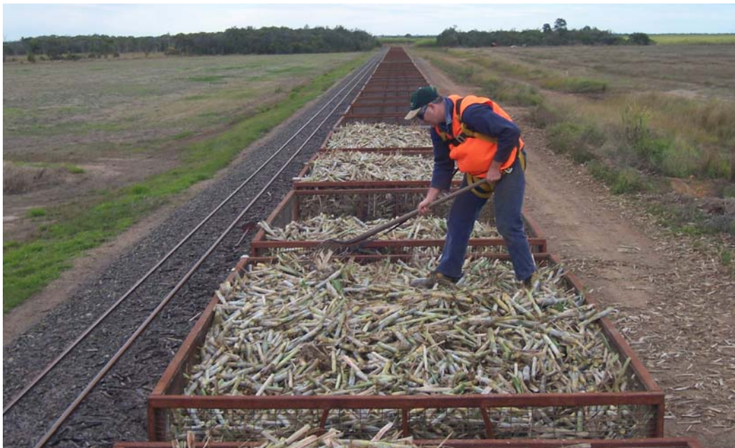
PHOTOGRAPH 8 - LEVELLING THE CANE IN EACH RAILWAY BIN TO DETERMINE BIN VOLUME
