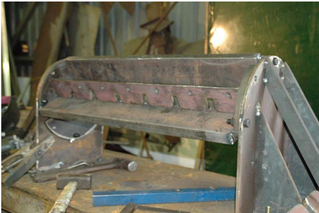
PHOTOGRAPH 2 - FABRICATION OF THE BOTTOM DRUM OF THE PROOF-OF-CONCEPT MODIFIED ROTARY-PINCH CHOPPER SYSTEM
