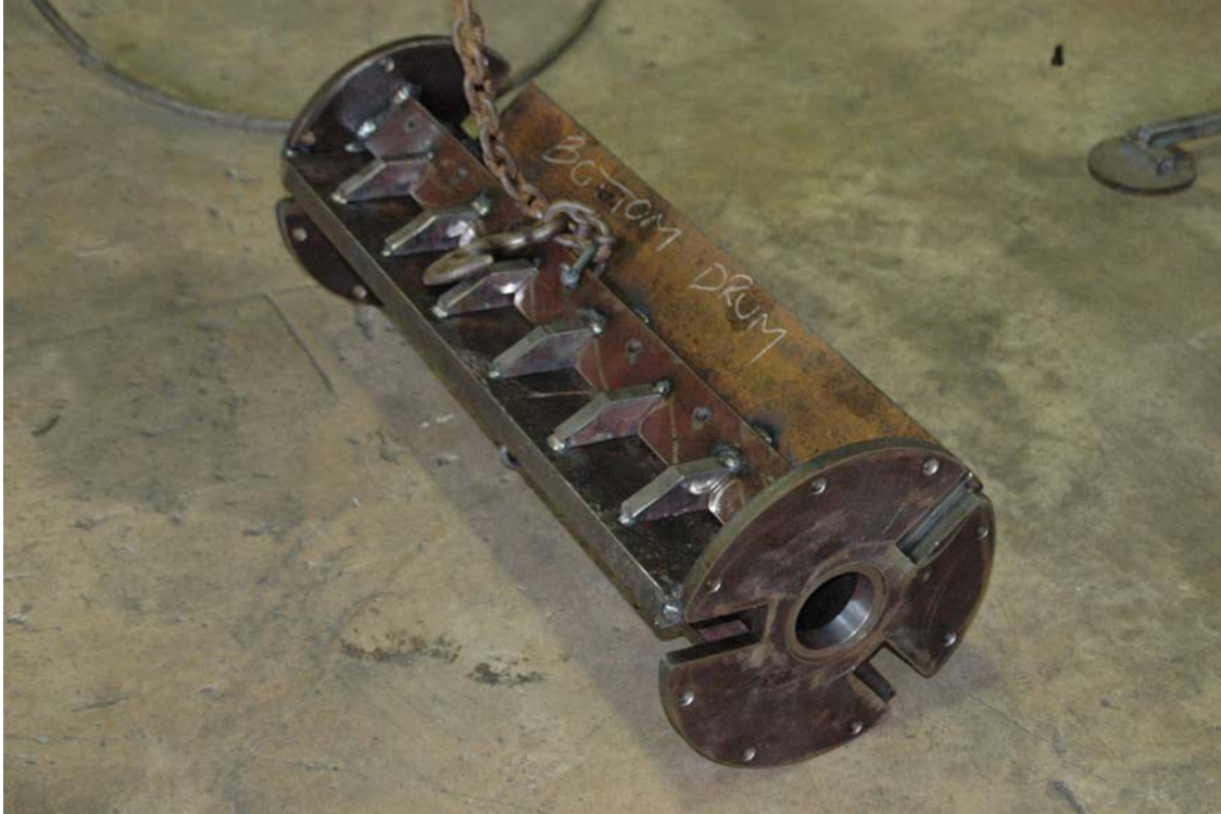
PHOTOGRAPH 3 - FABRICATED BOTTOM DRUM OF THE PROOF-OF-CONCEPT MODIFIED ROTARY-PINCH CHOPPER SYSTEM PRIOR TO MACHINING
