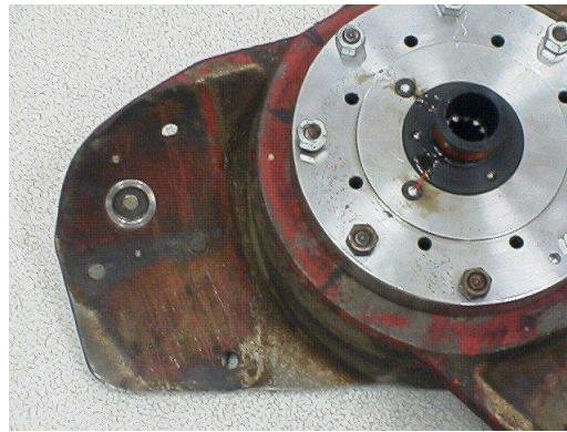
Figure 1: Acoustic transducer in extractor fan hub
