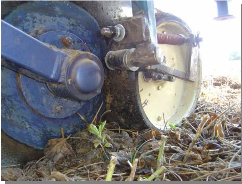
Photo 10. Press wheels mounted to the side of discs have reduced 'break-out
