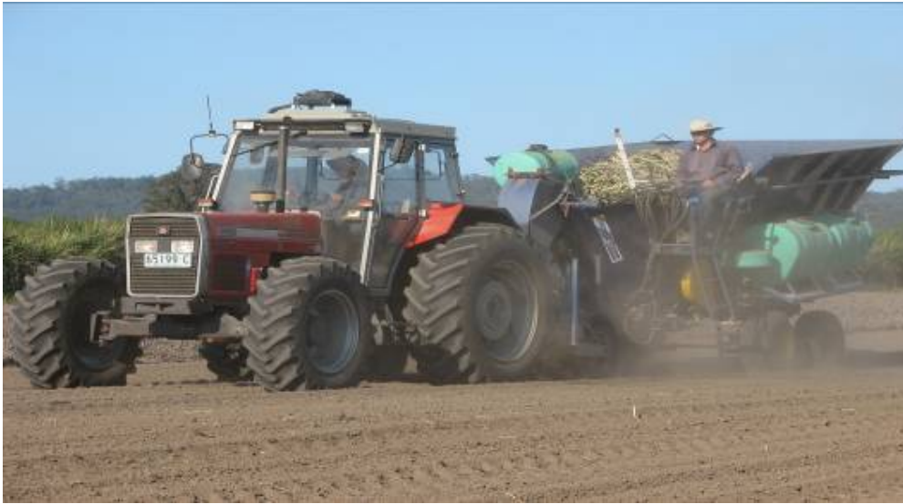
Photo 3: The Hodge double-disc-opener planter in action at Harwood.
