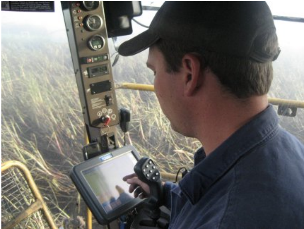
Photo 5: A harvester operator using GPS auto-steer.
