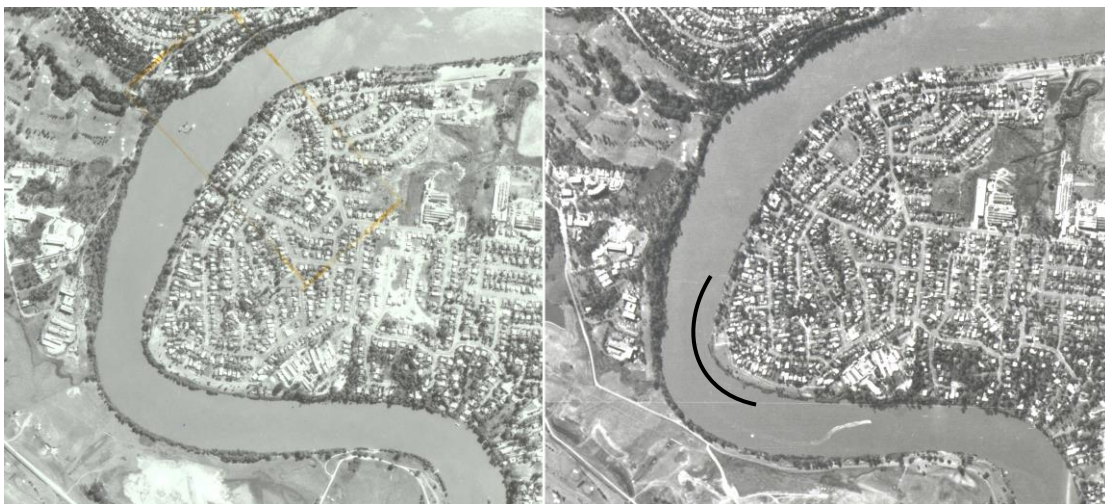
Figure 21. The Brisbane River at Long Pocket Reach in 1973 (left) and 1979 (right). The black line indicates areas of the river bank at Yeronga where mangroves disappeared or were reduced in extent between the two dates. (Aerial photographs supplied by NR&M).
