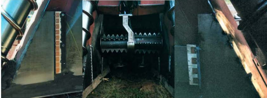
Figure 4.3 : Picture showing ground detection sensor mounted on the inside of the Austoft harvester row dividers.
