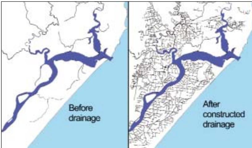
Figure 8. Natural and artificial drainage on a typical northern NSW floodplain. The amount of intact wetlands on coastal floodplains has been greatly reduced by drainage.
