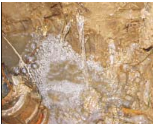
Figure 38. Acid groundwater flowing through large soil pores rapidly filling an excavated pit. Even though this acid sulfate soil has a clay texture, it has high hydraulic conductivity and rapid lateral movement of groundwater due to the network of interconnected pores and cracks. (Photo: Thor Aaso)
