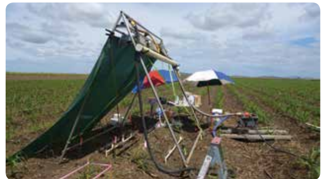
Above: Rainfall simulator being used to measure herbicide in runoff trials.
