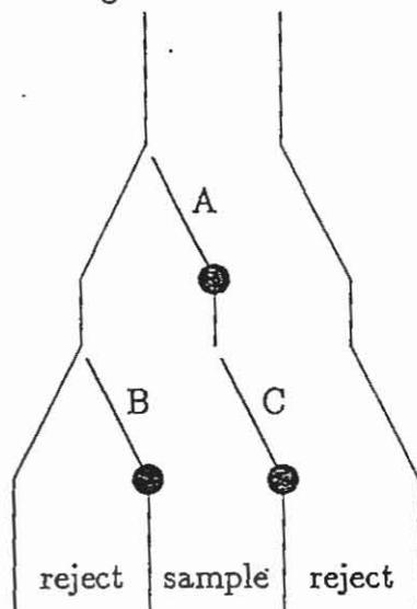
The reason why a subsampler designed this way is unbiased is that the motion which starts the sample is the same as that which ends the sample: flap A moving to the right.
