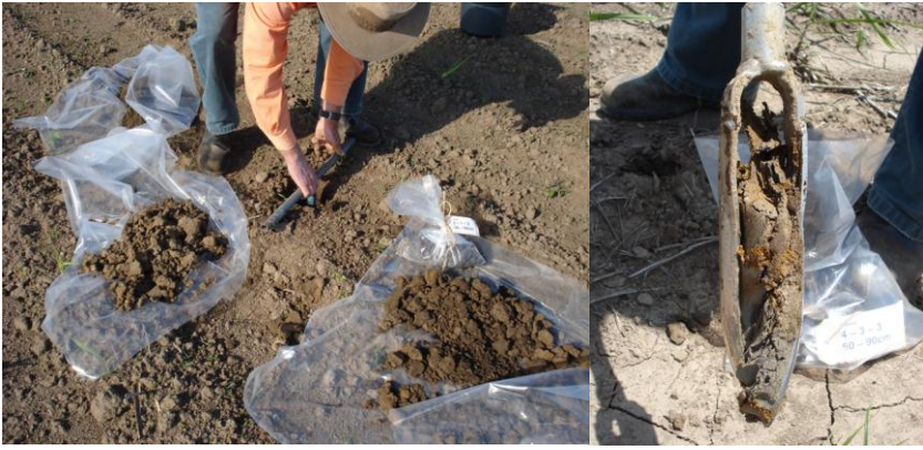
Plate 1. Soil at each trial site was sampled at six locations across the site and from three depth intervals: 0–25cm, 25–50cm and 50–90cm. Each depth interval was analysed separately. Photo: N. Moore NSW DPI
