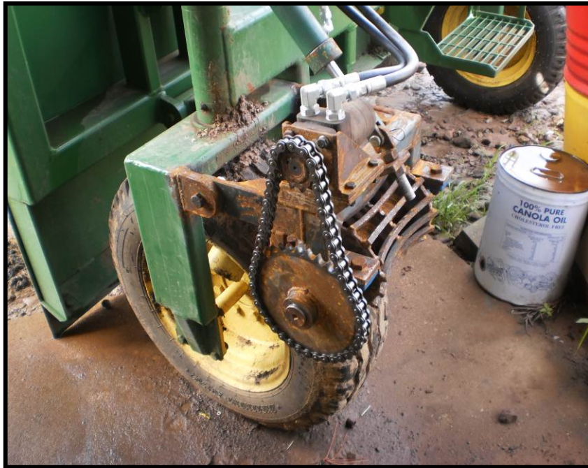
Figure 3. Hydraulic drive wheel assembly required to keep the machine running straight when mixing.
