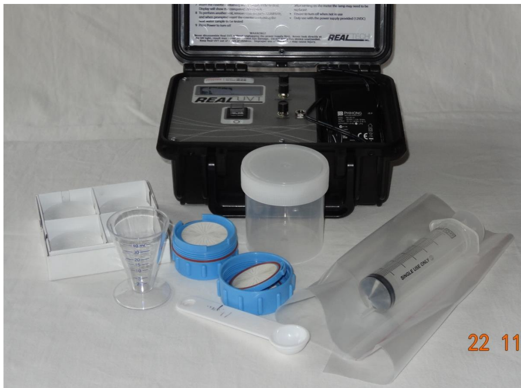
Figure 6: Components of the field UV method testing kit. From front left to right, 47 mm diameter, 45 \mu m glass fibre filter paper discs, 40 mL measuring cup, 47 mm filter disc holder, one teaspoon measure, one capped plastic container for shaking the solution, one 60 mL syringe for forcing the liquid through the filter, and a sealed plastic bag for pulverising the soil sample. Portable UV spectrophotometer is at the rear.
