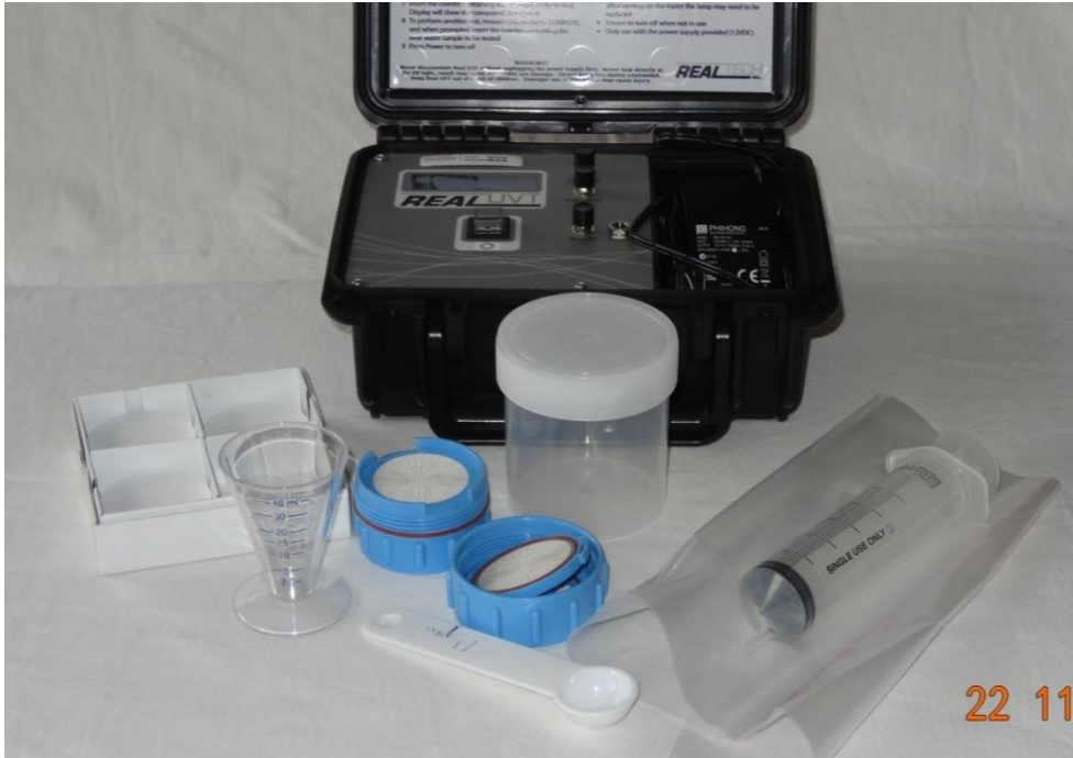
Figure 9: Components of the field UV method testing kit. From front left to right, 45 \mu\text{m} glass fibre filter paper discs, 40 mL measuring cup, filter disc holder, one teaspoon measure, one capped plastic container for shaking the solution, one 60 mL syringe for forcing the liquid through the filter, and a portable UV spectrophotometer is at the rear. Two capped vials for filtering the soil solution have not been included.
