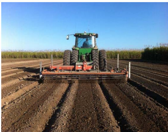
Figure 3. Zonal ripping and rotary Hoeing before planting on the pre-formed bed treatments- late July, 2012.
