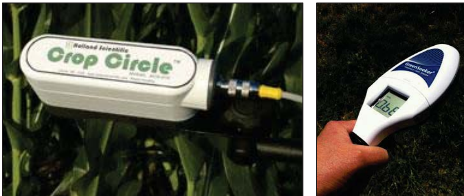
Figure 5.3. Two examples of AOS systems: (a) Crop Circle™ and (b) GreenSeeker. Source: Trotter and Lamb, (2013).
