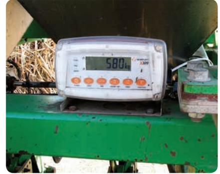
*A fertiliser box has been specifically developed for this project. It includes load cells that allow Julian to monitor the amount of fertiliser which has been applied to each strip. This piece of machinery is a stool splitter and side dresser. It is not common place to use a commercial size piece of equipment to undertake research. This is yet another factor that makes this project unique.*
