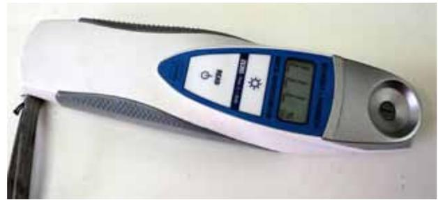
Figure 4: A refractometer with a digital readout.
