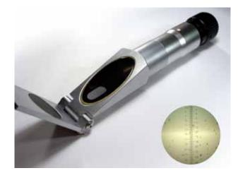
Figure 2: A refractometer.
