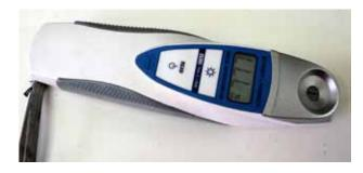
Figure 4: A refractometer with a digital readout.
