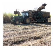
Measuring cane yield with commercial harvesters and weighing equipment. Sucrose and fibre content are analysed by Near Infrared Spectroscopy (NIR).
