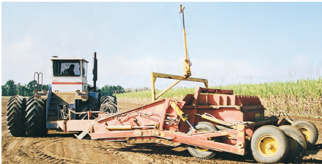
Figure 5. Laser levelling a cane field in the Ingham district.
