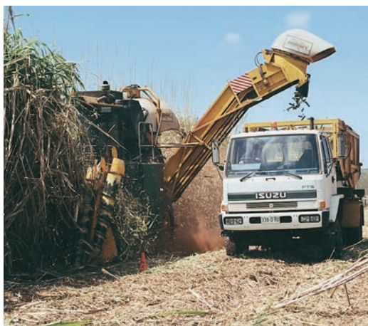
Figure 1. Green cane is harvested during trials using a weighing truck.
