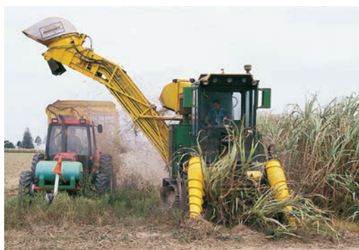
Figure 11. A four-row harvester has been developed to harvest cane planted under a close-row planting system.
