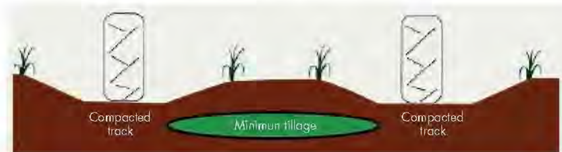
Figure 4. Schematic view of dual rows in a controlled traffic/minimum tillage system.
