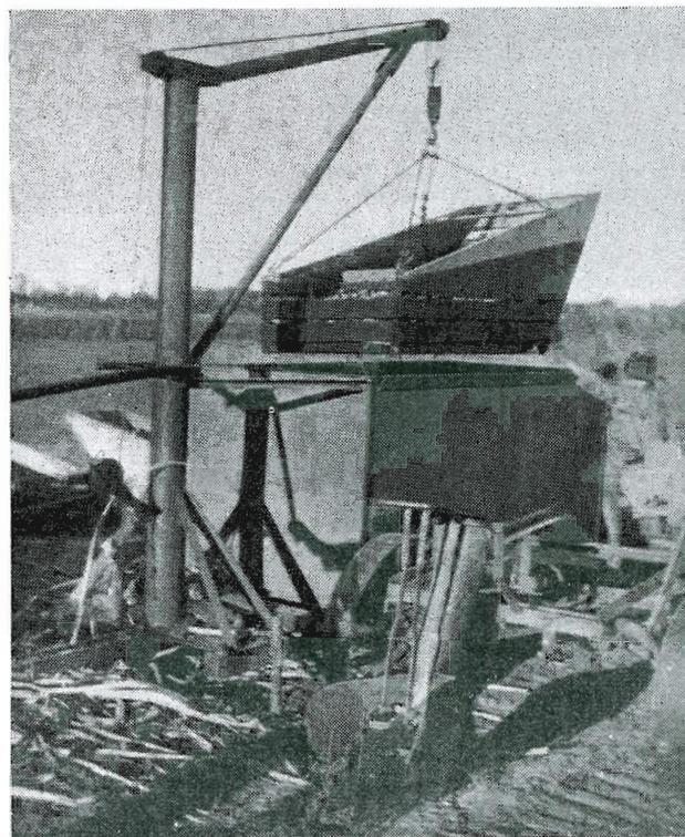
FIG. 7.—Large dipping plant, showing full detachable planter-box draining after immersion in solution.
