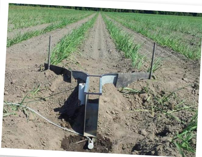
**Left:** The flumes that measure N loss through the irrigation events on the farm.
