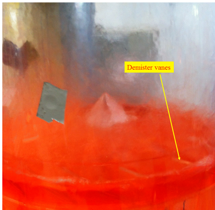
Fig 10 – Part view of the scrubber scale model showing the water overflowing into the region above the demisting vanes when the air flow is very high.
