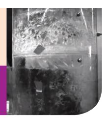
Queensland University of Technology (QUT) researchers have used a scale-model of a wet scrubber to provide valuable information for sugar millers on how this piece of milling equipment functions – and to recommend possible modifications and improvements.
