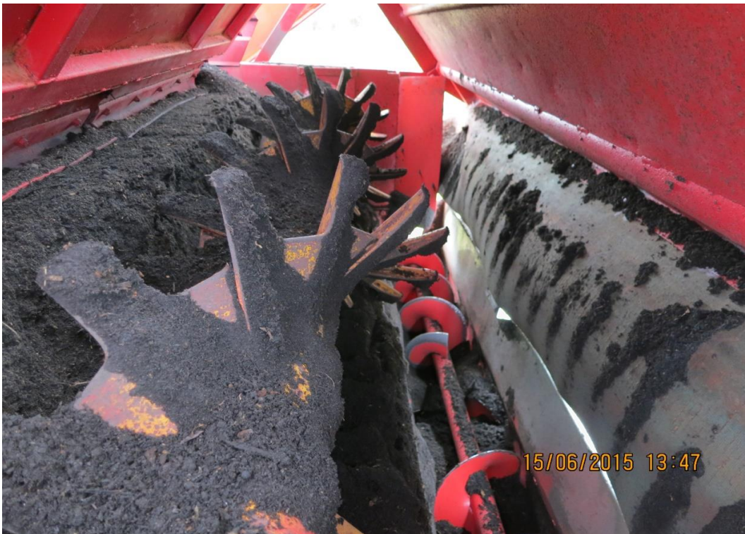
Photo 3 – The agitator system ensures a consistent flow into the feeder.
