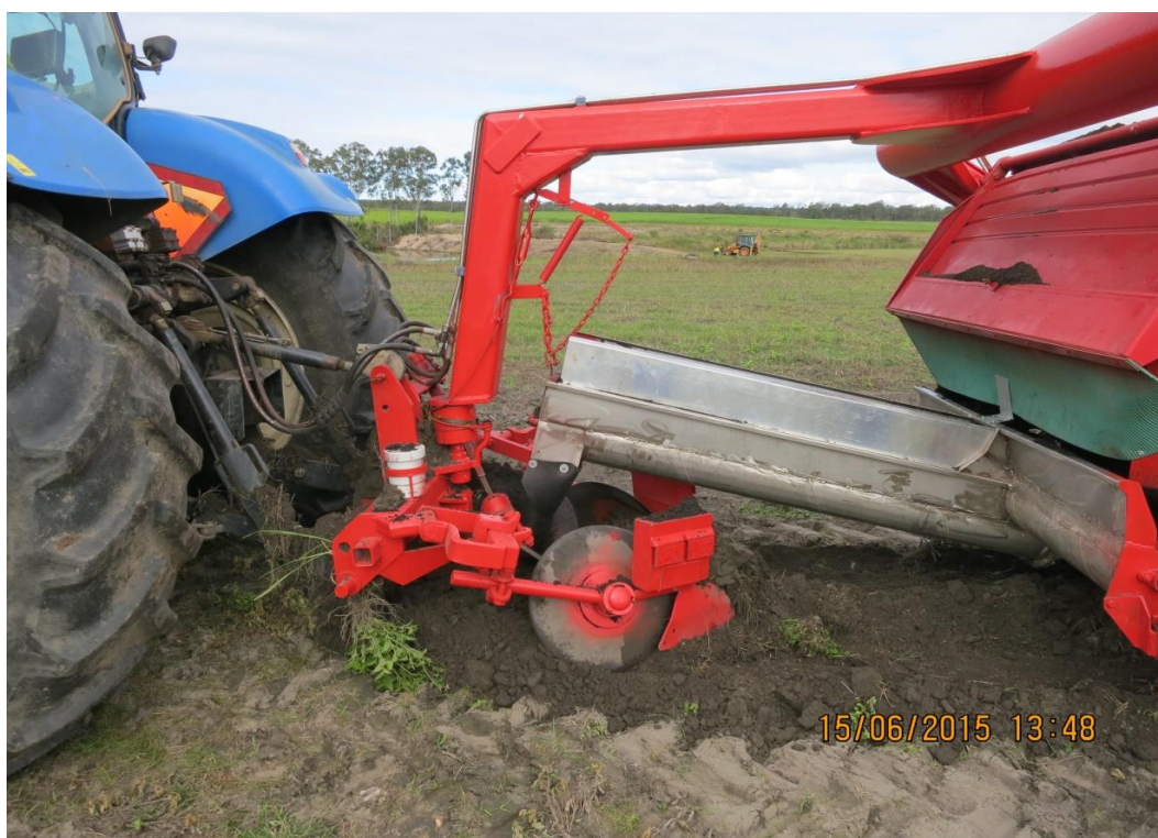
Photo 1 – Covering discs and feeder shoot. The covering discs leave a bed with a curved row profile that is appropriate for harvesting.
