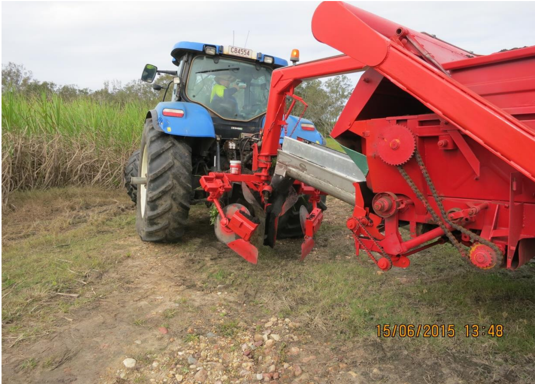
Photo 2 – The goose neck assembly allows the machine to turn on narrow headlands
