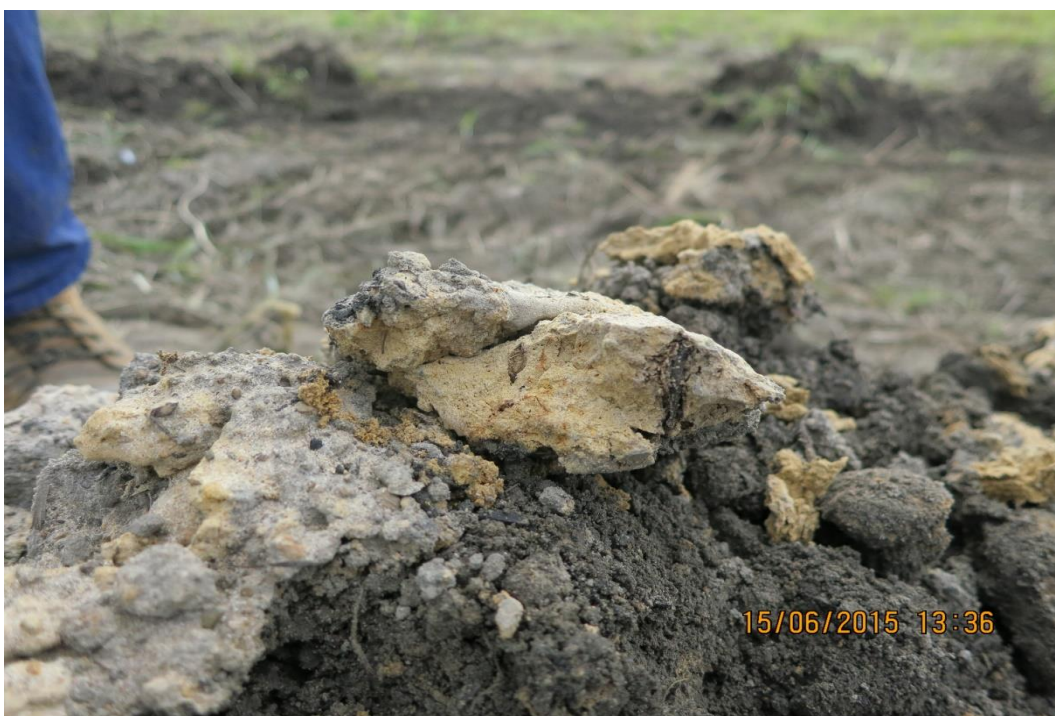
Photo 5 – Clay sub soil from the MSF demo site after 10mm of rain, note how the clay has dispersed and the surface has “hard set”.
