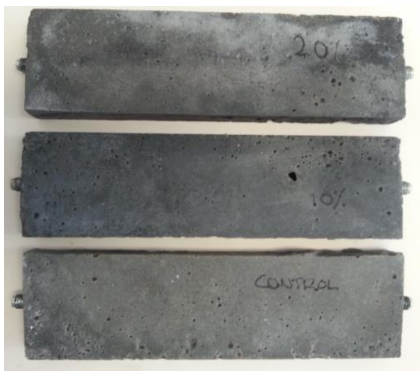
Figure 15. Mortars with 20% (top) 10% (middle) and 0% (bottom) SCBA replacing OPC exposed to sulphate solution at 2 weeks.
