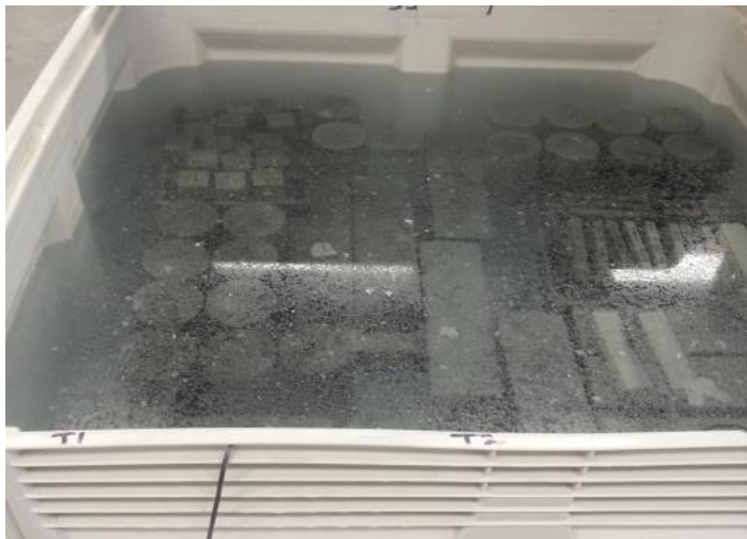
Figure 6 Concrete and mortar specimens in the lime saturated curing tank.
