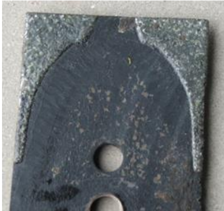
Figure 8.6 Basecutter blade showing a thin layer of hardfacing on the underside of the blade.
