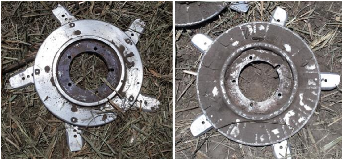
Figure 8.7 Basecutter disc with angled back blades on the left and the standard configuration on the right.
