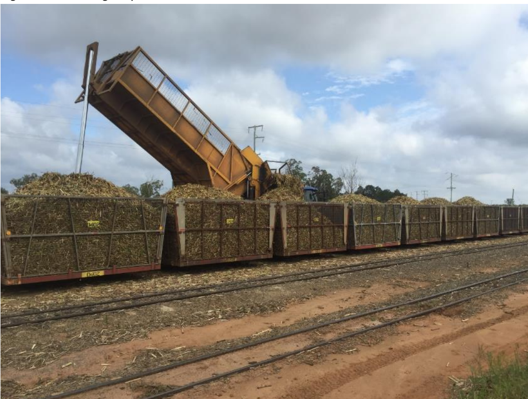
Figure 43 The 'McLean' bin that allows for topping up of bins
