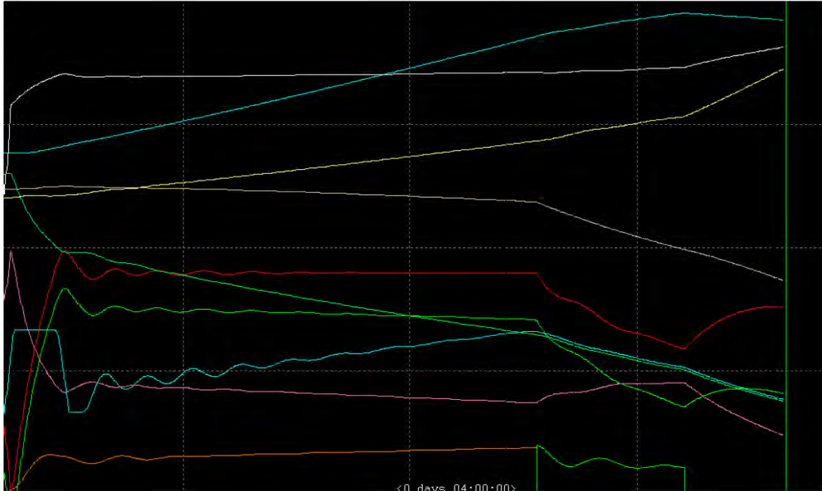
Figure A.6 Trends for A massecuite boiling with 100 kPa abs vapour supply, syrup at 72 dry substance and syrup and A molasses supplied at 70 °C
