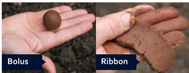
The textural grade of a soil is a function of its relative amounts of sand, silt and clay. It can be deduced by the length of the unbroken ribbon resulting from squeezing some moistened soil (bolus) between the thumb and forefinger.
