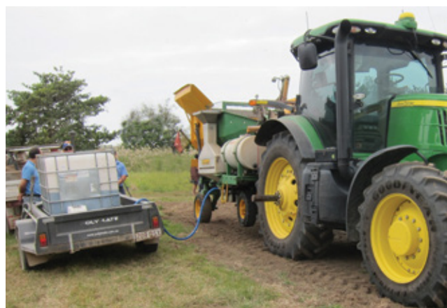
Sugarcane billet planter and liquid fertiliser applicator. Pumping fertiliser into application tank.
