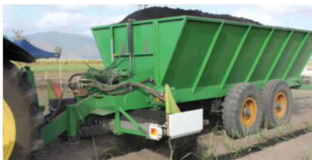
Much lower application rates of mill by-products are possible with precision-application equipment.
