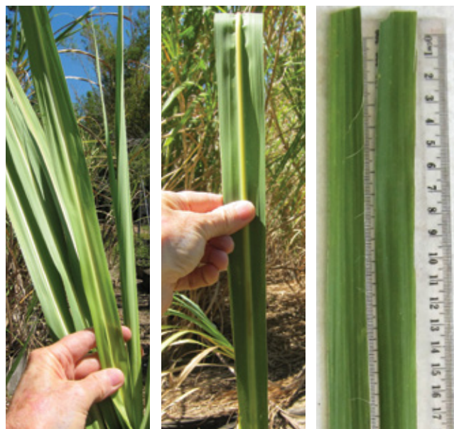
Leaf analysis samples comprise the third unfurled or partially unfurled leaf (left). The middle 200 mm section of 20 - 30 leaves is selected (centre), the midrib is removed (right), and the leaf blades are dried and sent to the laboratory.
