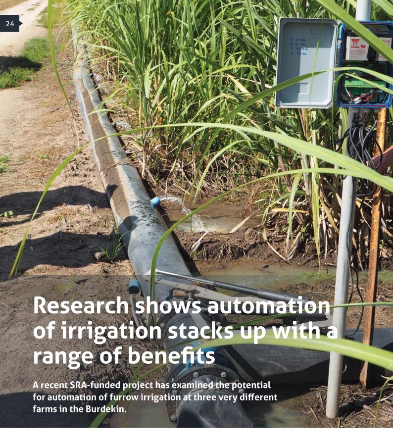
The National Centre for Engineering in Agriculture (NCEA) received funding from SRA to investigate the automation of furrow irrigation in the sugar industry. This involved a review of potential commercially available control hardware, sensors and radio systems and the installation of this equipment on three farms. These farms were chosen because they represented
